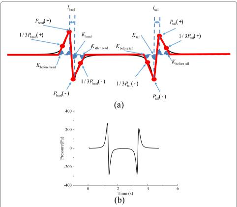
**Fig. 10** Wind pressure curve model of bottom plate: **a** simplified diagram of a-di-1 wind pressure curve; **b** wind pressure time history curve of bottom plate
