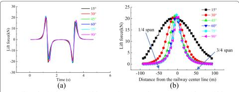
**Fig. 9** Effects of angle of intersection: **a** lift force time history curve; **b** attenuation curve of positive lift force of head wave along longitudinal bridge direction
