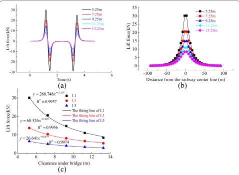
**Fig. 8** Effects of clearance under bridge: **a** lift force time history curve; **b** attenuation curve of positive lift force of head wave along longitudinal bridge direction; **c** variation of positive lift force extremum of head wave in L1, L3, L5 with train speed
