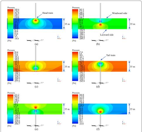
**Fig. 6** Wind pressure nephogram: **a** nose of head carriage reaches the windward side; **b** nose of head carriage reaches the center line of the girder; **c** nose of head carriage reaches the leeward side; **d** nose of tail carriage reaches the windward side; **e** nose of tail carriage reaches the center line of the girder; **f** nose of tail carriage reaches the leeward side
