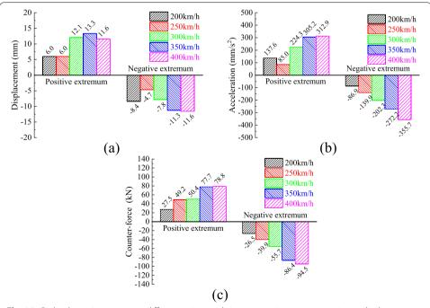
**Fig. 14** Girder dynamic response at different train speeds in construction stage: **a** maximum displacement value; **b** maximum acceleration value; **c** maximum counter-force of the temporary pier
