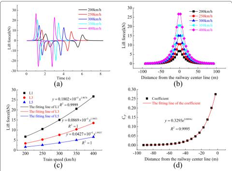
**Fig. 7** Effects of train speeds: **a** lift force time history curve; **b** attenuation curve of positive lift force of head wave along longitudinal bridge direction; **c** variation of positive lift force extremum of head wave in L1, L3, L5 with train speed; **d** head wave lift force positive extremum coefficient along longitudinal bridge direction
