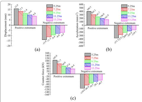
**Fig. 15** Girder dynamic response at different clearances under bridge in construction stage: **a** maximum displacement value; **b** maximum acceleration value; **c** maximum counter-force of the temporary pier
