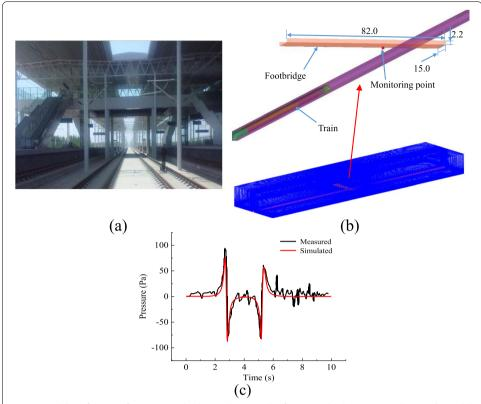
**Fig. 2** Model verification of an overpass bridge: **a** photograph of overpass bridge (Yang et al. 2015); **b** model of high-speed train crossing under overpass bridge (unit: m); **c** comparison of simulated and measured wind pressure
