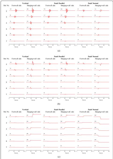
**Fig. 5** Simulation results of the low-frequency ground motion time histories at each bridge site: **a** acceleration; **b** velocity; **c** displacement. The number of each subplot indicates the peak value with the unit in cm/s<sup>2</sup>, cm/s and cm for acceleration, velocity and displacement, respectively. The numbers on the left correspond to the bridges listed in Table 1
