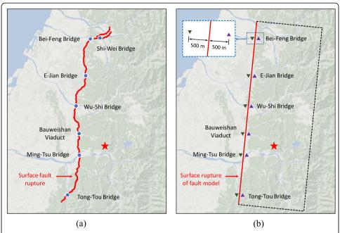
**Fig. 3** Plan view of the fault-crossing bridges in the 1999 Chi-Chi earthquake: **a** real bridge locations; **b** observation points for ground motion simulation. The red lines indicate the surface fault rupture; the red star indicates the epicenter; the dashed rectangle indicates the projection of the fault model on the ground surface; and the upward and downward triangles represent the simulation locations on the hanging-wall and footwall sides, respectively
