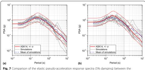
**Fig. 7** Comparison of the elastic pseudo-acceleration response spectra (5% damping) between the simulated horizontal across-fault ground motions and the GMPE ASK14: **a** Footwall side; **b** Hanging-wall side
