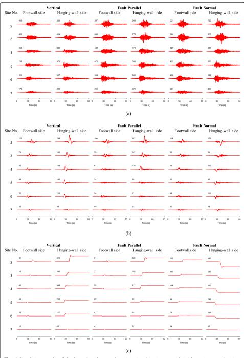
**Fig. 6** Simulation results of the broadband ground motion time histories at each bridge site: **a** acceleration; **b** velocity; **c** displacement. The number of each subplot indicates the peak value with the unit in cm/s², cm/s and cm for acceleration, velocity and displacement, respectively. The numbers on the left correspond to the bridges listed in Table 1
