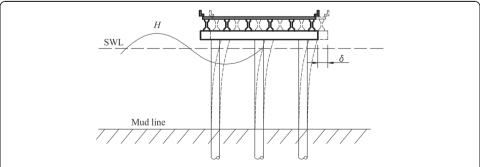
**Fig. 1** Schematic diagram for the bridge deck-wave interaction under extreme waves. H is the wave height;  $\delta$  is the motion displacement of the bridge deck; SWL refers to the still water level
