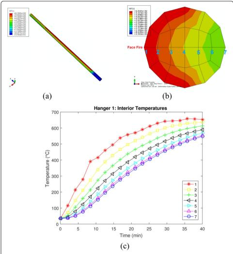
**Fig. 4** The thermal analysis illustration for the baseline case: **a** the whole hanger model; **b** the internal temperature distribution over the cross section at height 300 cm at 24 min; **c** time histories of interior temperature of different nodes within the same cross section
