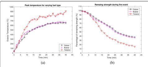
**Fig. 12** Comparison of peak exterior temperatures and remaining strengths of the hanger with different gasoline surrogates (10 m/s wind speed): **a** peak exterior temperature; **b** percentage of remaining strength based on ASCE code
