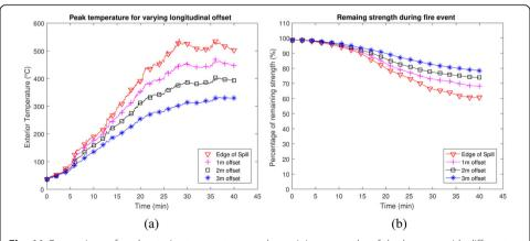
**Fig. 11** Comparison of peak exterior temperatures and remaining strengths of the hangers with different longitudinal offset distances from edge of fire (10 m/s wind speed): **a** peak exterior temperature; **b** percentage of remaining strength based on ASCE code
