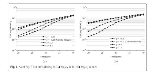
can be seen that a greater variation of the live load results in a larger failure probability for the bridge. Correspondingly, with the same target reliability, the predicted service life is shortened by LL2. The impact of the deterioration model on structural failure probability, however, is similar to the observations in Fig. 2.
