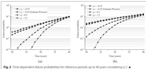
**Fig. 2** Time-dependent failure probabilities for reference periods up to 40 years considering LL1. **a**  $\sigma_{G(40)} = 0.14$ ; **b**  $\sigma_{G(40)} = 0.21$
