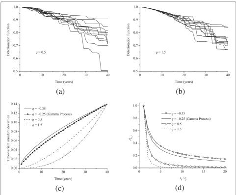
**Fig. 1** Illustration of the proposed resistance deterioration model. **a** and **b** Sampled deterioration trajectories; **c** Time-variant standard deviation with different values of q; **d** Autocorrelation coefficient with different values of a
