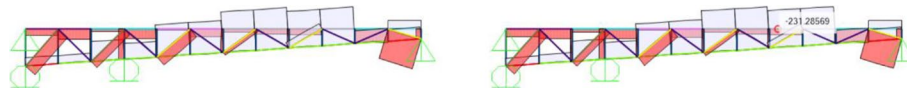
Fig. 35 Member forces (KN) for scenario IV and scenario V in the left truss
