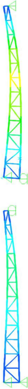
Fig. 26 Deflection of truss for scenario I case A (left) and case B (right)
