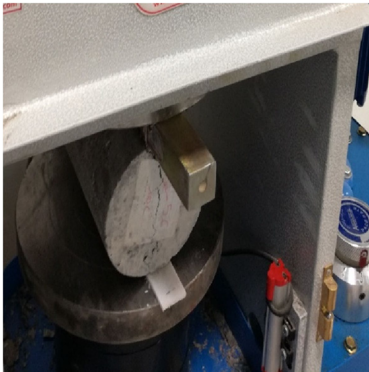
Fig. 11 Cylindrical sample inside the concrete breaker
