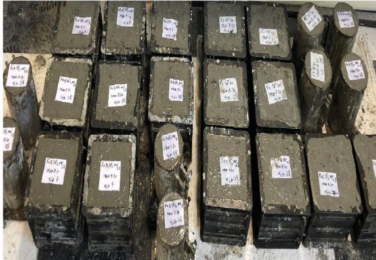
Fig. 7 Concreting in standard forms
