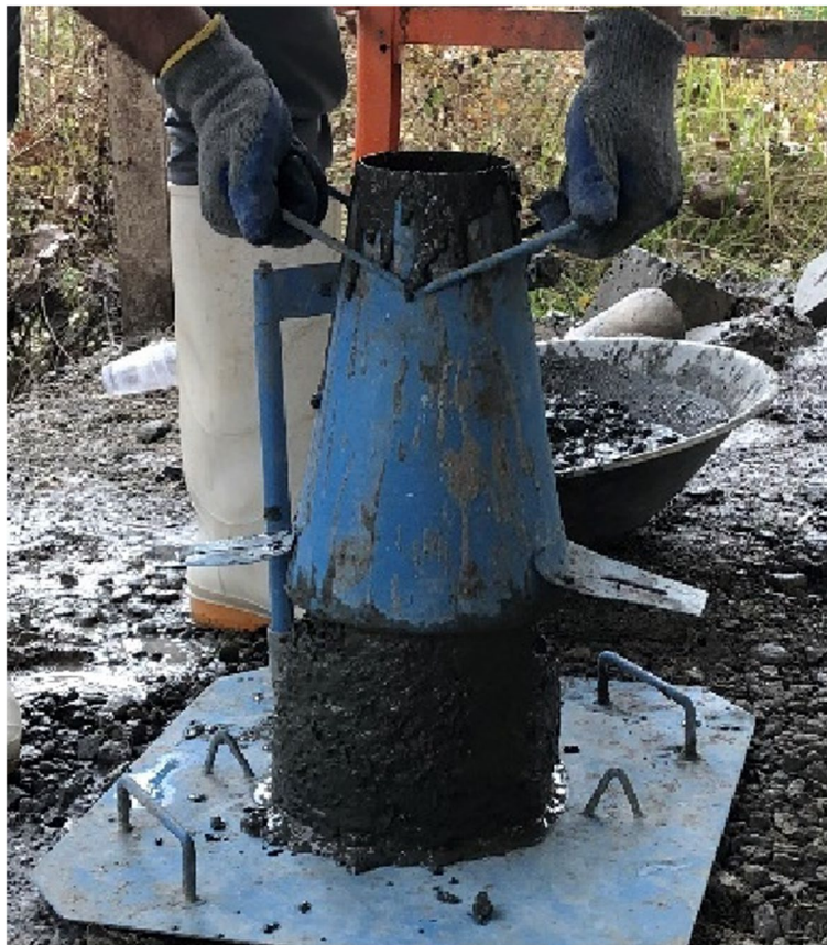
Fig. 9 Concrete slump test
