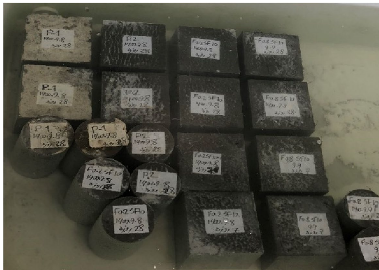
Fig. 8 Samples made during processing in the water basin
