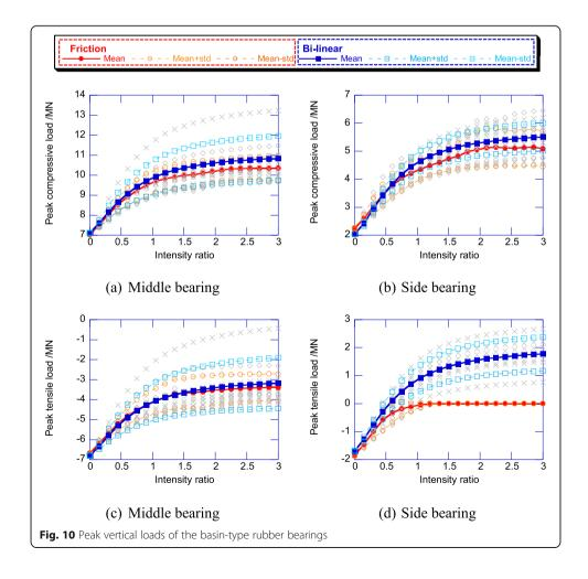
bearings were not consistent. For middle bearing under *IR* equaling to 3.0, the maximum vertical load was about 1.51 times of the gravity load. While side bearing subjected to 2.54 times of the gravity load under the same *IR*.
